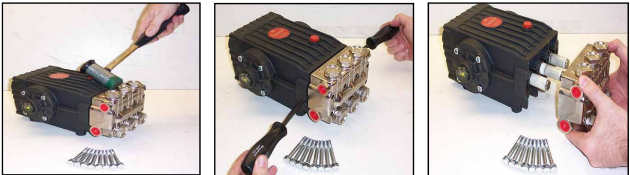
Figure 5-6. Separate Manifold from Crankcase
