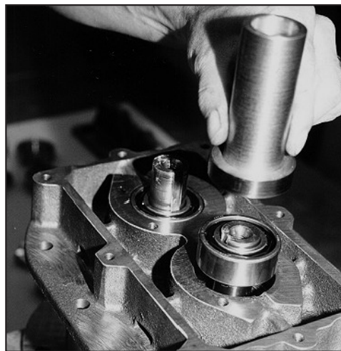
Figure 10. Tapping Bearings into End Plates
