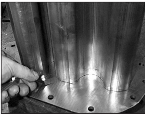
Figure 11. Checking Gear End Clearances
