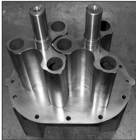
Figure 9. Rotors Assembled on Drive End Plate (Model 4000 with tri-lobe rotors shown)
