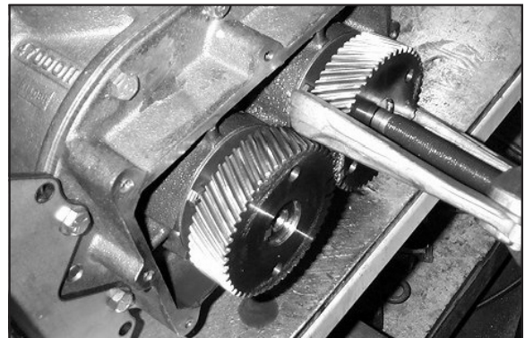
Figure 2. Pulling Driven Gear with Jaw Puller
