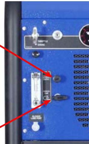
Figure 4-3. Location of Chemical Metering Control and Chemical Pump Selector Valve
