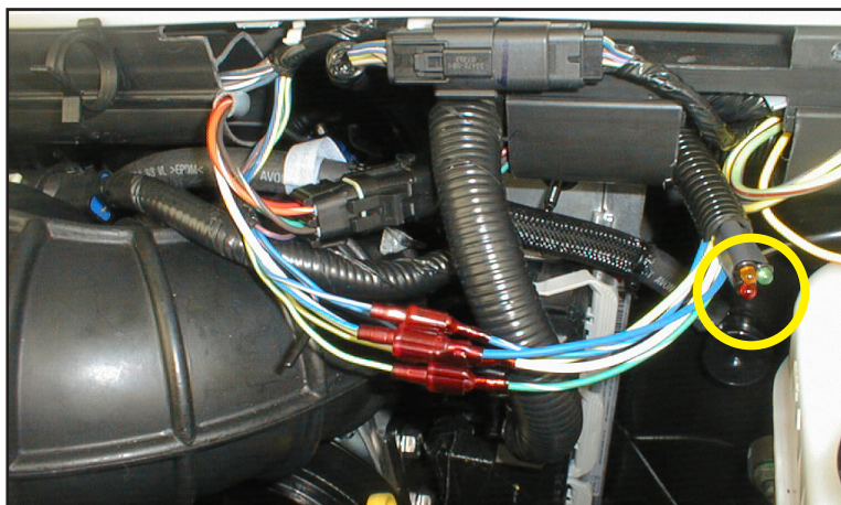
Figure 3-2. Location of 3 Lights on Throttle Control Assembly
