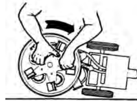
Figure 6-3. Loosen Cleaning Head Assembly
